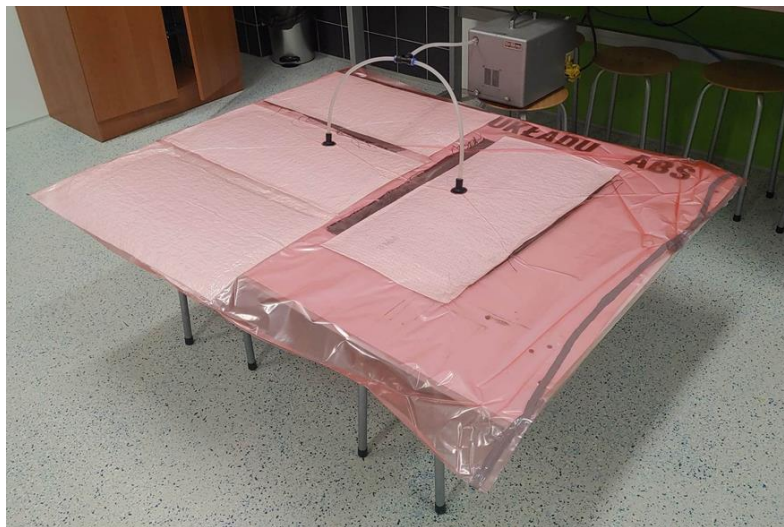
Fig. 2. Lamination of glass fibre-reinforced aluminium laminates.
