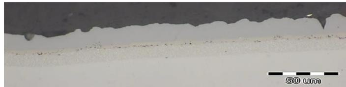
**Fig. 2.** Microstructure of the aluminized layer; non-etched microsection treated with Kalling's reagent (blade's suction side).
