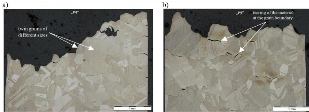
**Fig. 12.** Cross-sectional view of the zone adjacent to the fracture of the a) P4 sample b) P9 sample. In the structure, twin grains of different sizes and typical effects of the creep process (tearing of the material at the grain boundary) are visible. Etchant: Kalling's reagent.
