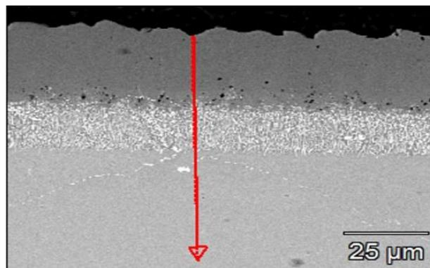
**Fig. 5.** a) Linear profile of changes in the content of elements along a given scanning line on b) the cross-section of a blade with an aluminide layer produced in the aluminizing process using the "above the pack" method.
