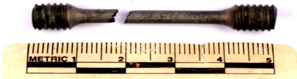
**Fig. 10.** Sample cut from the P4 blade - the sample after the creep resistance test broke after 42.6 h.
