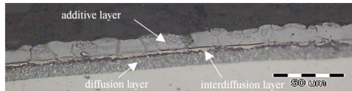
**Fig. 1.** Microstructure of the aluminized layer showing the in gray and orange; non-etched microsection of the blade's suction side.
