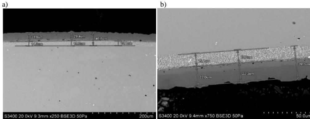
Fig. 4. Microstructure of the aluminide layer formed in the thermochemical process ("above the pack" method): a) suction side, b) pressure side – leading edge. The depth of the layer is indicated.
