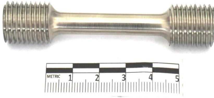
Fig. 7. Appearance of the sample used for creep resistance testing.
