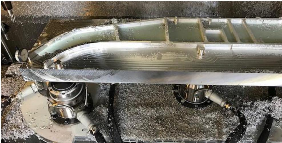
**Fig. 4.** Milling test performed on the CNC machine - operation OP10.
