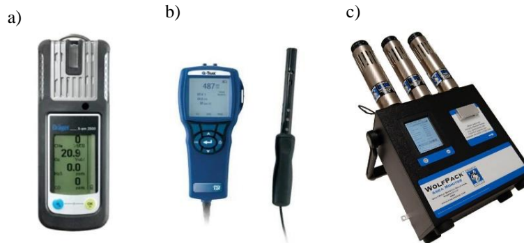
Fig. 1. Measuring instruments used in the field survey of pollutant samples: a) Dräger X-am 2000 gas detector, b) air quality monitor model TSI Q-Trak Model 7565 and c) GrayWolf meter for indoor air quality (IAQ) measurements.
