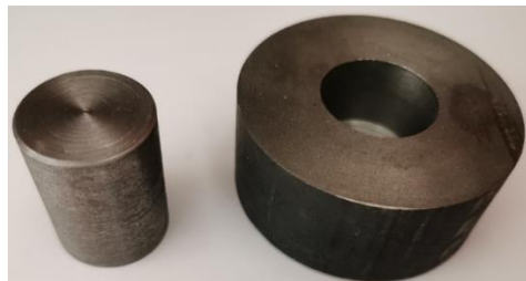
Fig. 2. Container and punch used in the volumetric compression tests.
