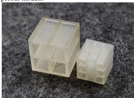
Fig. 2. 3D-printed porous structures; right: Model 1 and left: Model 2.
