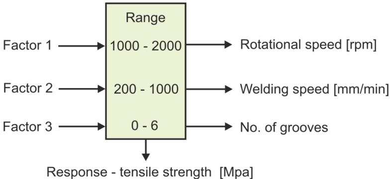
Fig. 4. Ranges of changes in welding parameters
