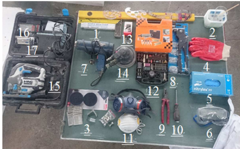
Fig. 2. Basic equipment required, set № 4 of 4: 1 – measuring equipment, 2 – resin mixing cup 50 l 8 bar, 3 – mechanical connections for bolide parts, 4 – chemical protective gloves, 5 – latex gloves, 6 – protective glasses, protective clothes and clean wipes, 7 – heating fan, 8 – rivet gun, 9 – pliers, 10 – manual screwdriver, 11 – dust particle protective mask FFP1 type and Moldex® type chemical, 12 – pneumatic grinding machine and basic attachments, 13 – pneumatic grinding machine specific round cutting abrasive for steel, 14 – pneumatic elliptical grinding machine, 15 – electric jig saw, 16 – standard blades for jig saw, 17 – abrasive blades for jig saw
