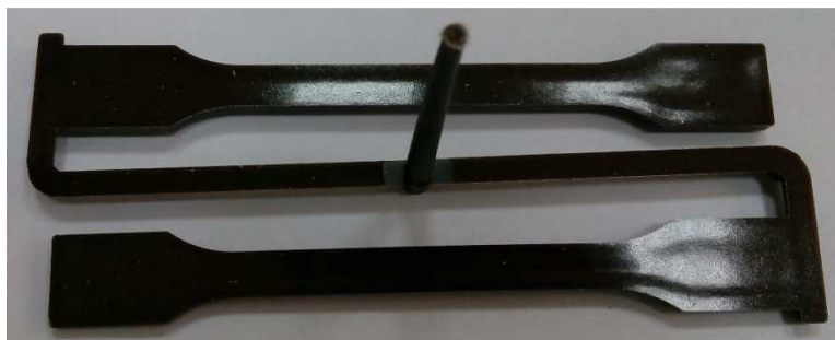
Fig. 4. The moulded piece made of composite PHBV-hemp fibres (fibre content: 15% by weight)
