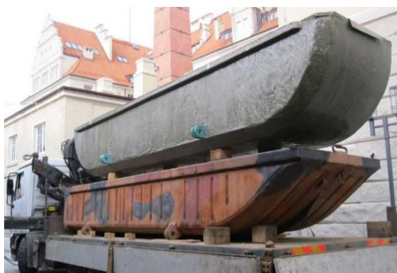
Fig. 4. Two pontoons, PP-64 at the bottom and the prototype made from composites at the top
