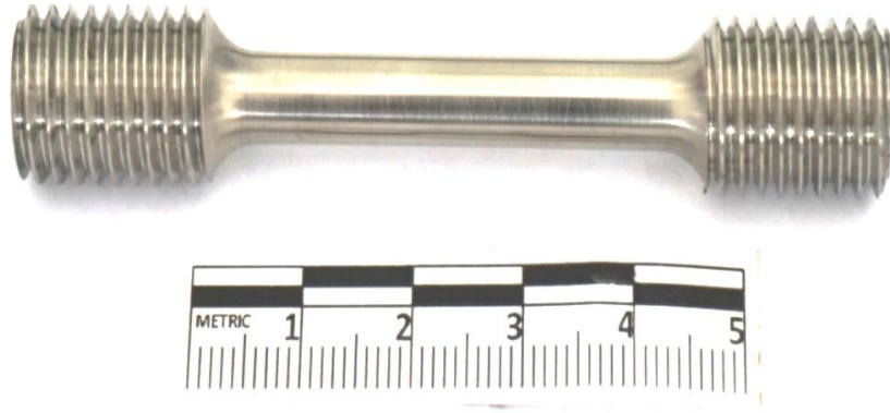
Fig. 7. Appearance of the sample used for creep resistance testing.
