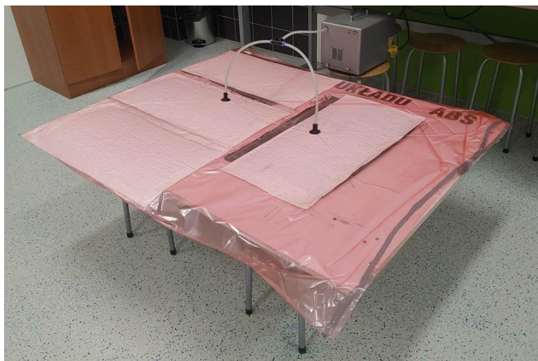
Fig. 2. Lamination of glass fibre-reinforced aluminium laminates.
