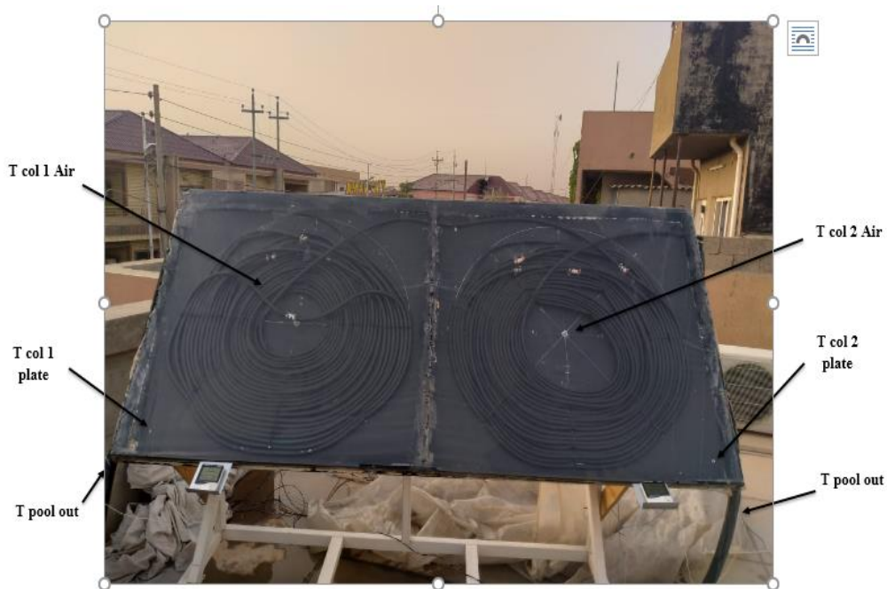
Fig. 6. Solar collector and thermocouple sensor location.
