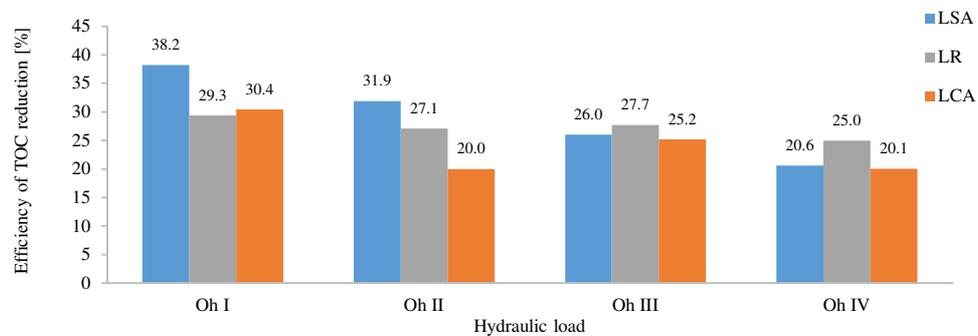
Fig. 7. The efficiency of TOC reduction depending on the filling material and hydraulic load – filtration process without aeration
