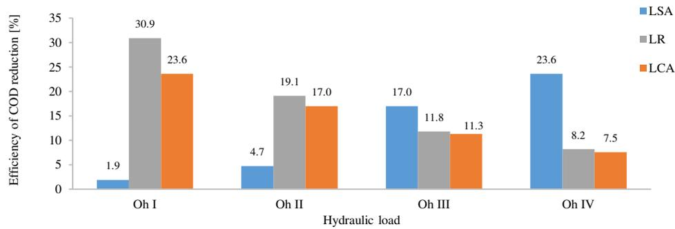
Fig. 6. The efficiency of removing organic compounds, determined by the COD, depending on the filling material and the hydraulic load – filtration process without aeration
