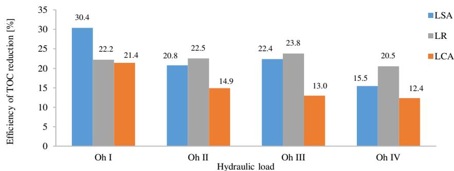
Fig. 3. Effectiveness of TOC reduction depending on the filling material and hydraulic load – filtration process with aeration
