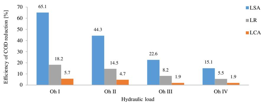
Fig. 2. The efficiency of removal of organic compounds, determined by the COD, depending on the filling material and hydraulic load – filtration process with aeration
