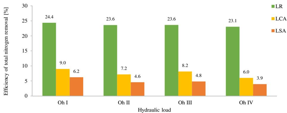
Fig. 8. Effectiveness of total nitrogen removal depending on the filling material and hydraulic load – filtration process without aeration
