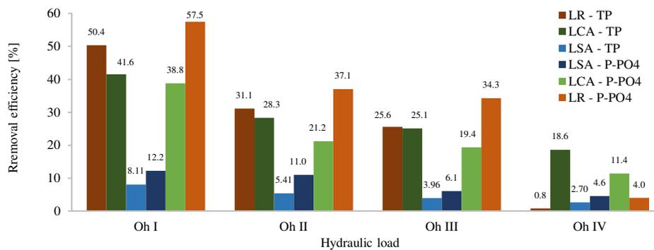
Fig. 5. Effectiveness of phosphorus compounds removal depending on the filling material and hydraulic load – filtration process with aeration
