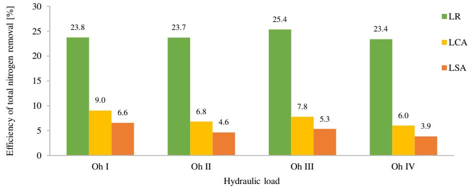
Fig. 4. Effectiveness of total nitrogen removal depending on the filling material and hydraulic load – filtration process with aeration
