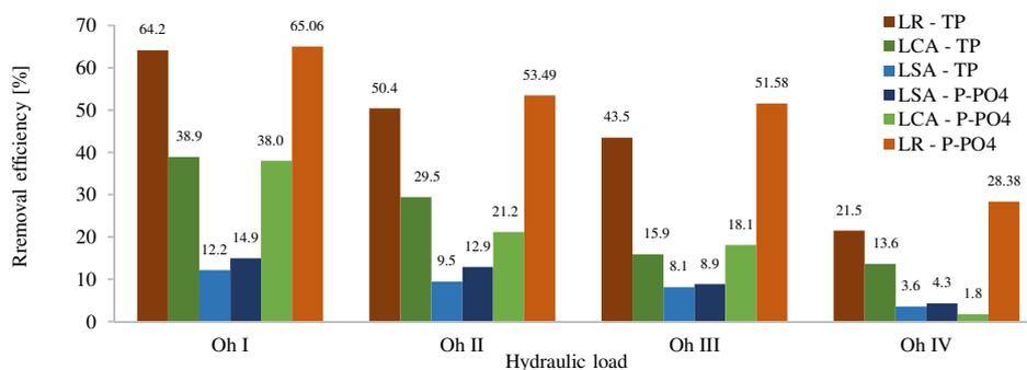
Fig. 9. Effectiveness of removing phosphorus compounds depending on the filling material and hydraulic load – filtration process without aeration
