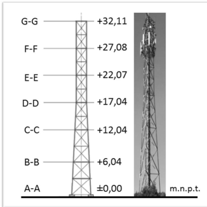
Fig. 1. View and scheme of arrangement telecommunication tower segments
