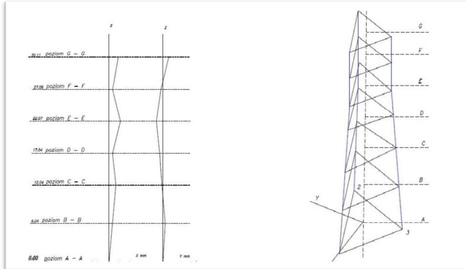
Fig 3. Graphs of the deviations of the tower axis from the vertical
