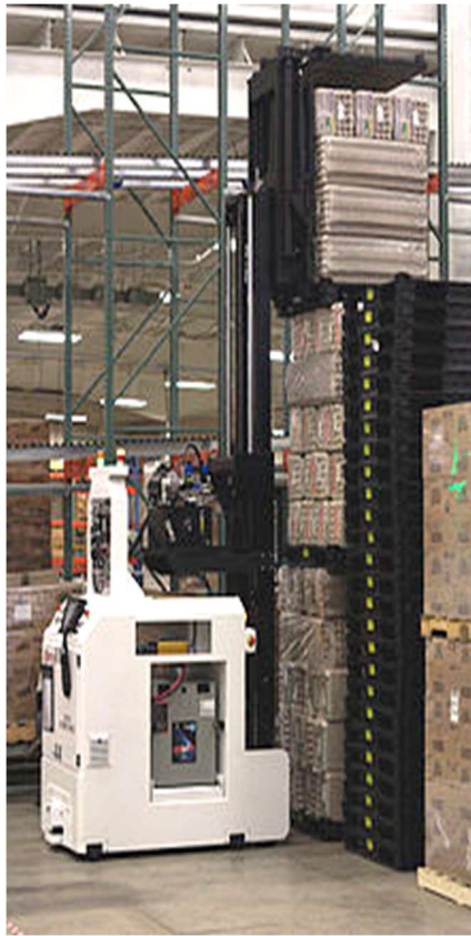
Figure 5. Forklift AGV with StabilizerPad. Source: (Wikipedia)
