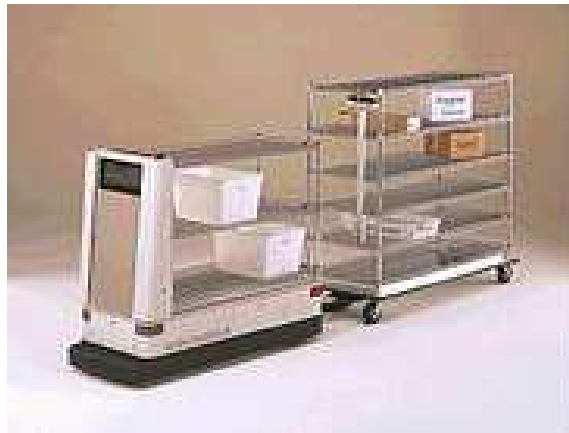
Figure 1. Example of a Packmobile with trailer, typical existing AGV Source: (Wikipedia).
