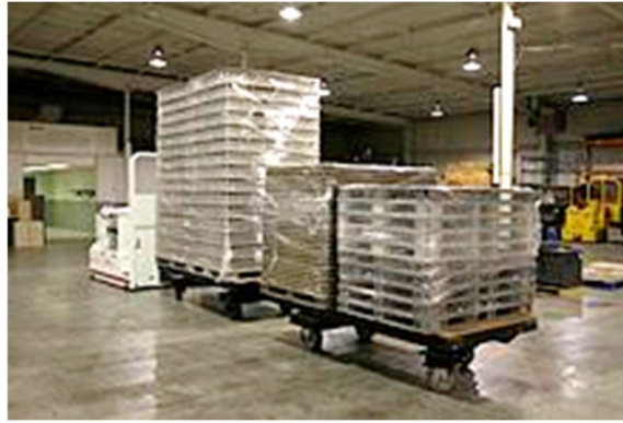
Figure 3. Tugger AGV towing multiple trailers in a warehouse environment Source: (Wikipedia).
