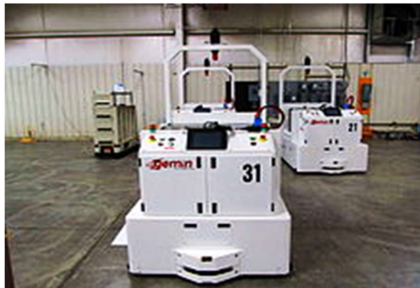
Figure 2. Tugger AGVs can move trailers or trains of trailers more safely than a manually operated tugger
