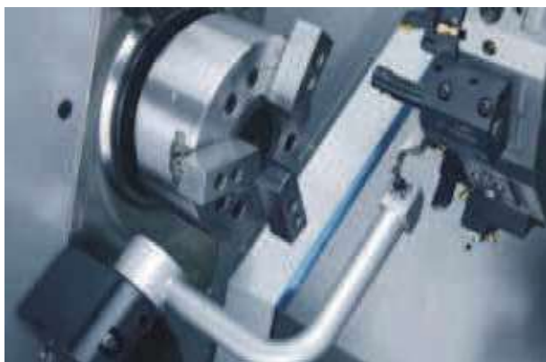
Fig. 5. Measuring probe of the lathe [10] Rys. 5. Sonda pomiarowa tokarki [10]
