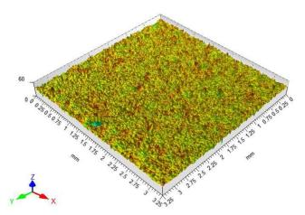
Figure 2. An example of surface morphology of the flexible adherend after sand blasting process
