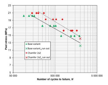
Figure 6. Comparison of the fatigue curves for the base variant and chamfer  $2 \times 2$  variant
