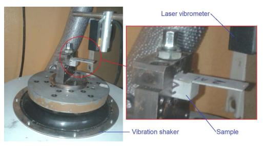
Figure 4. Setup for fatigue testing of adhesive joints
