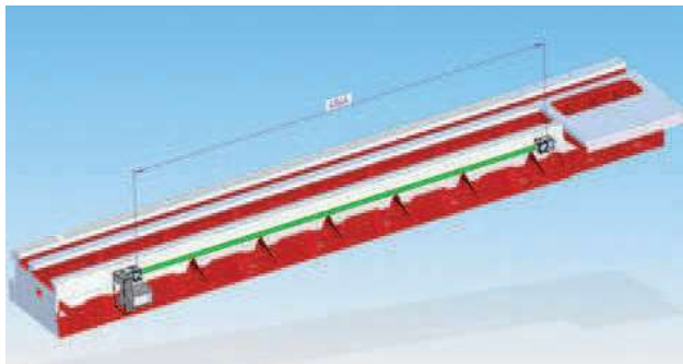
Rys. 4. Śruba bez podparcia Fig. 4. Ballscrew with no support
