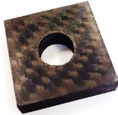
Fig. 6. Cube cut out of 7.3 mm thick composite
