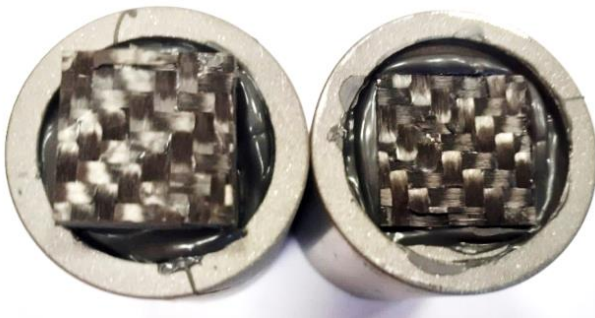
Fig. 5. View of the specimen after testing the strength of the composite in the x_3 direction
