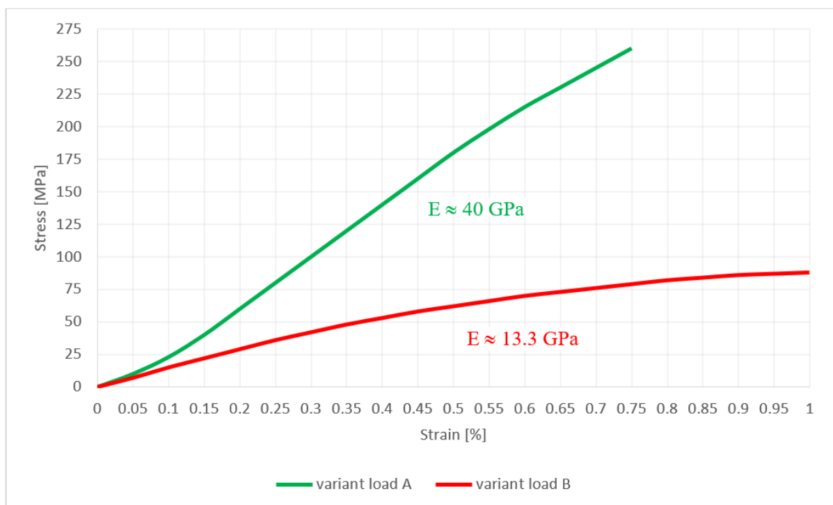
Fig. 9. Curves \sigma = \sigma(\epsilon) of composite No. 2
