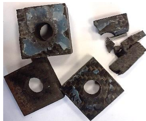
Fig. 13. The form of destruction of a compressed specimen element
