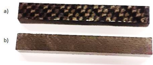
Fig. 7. Specimens for impact tests a) in the plane of laying composite layers b) in the cross-sectional plane of the composite
