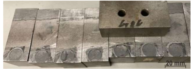
Fig. 12. Cohesive destruction of Raex 400 material samples with a diameter of 12.6 mm
