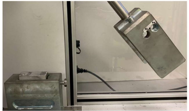
Fig. 6. Hammer prior to sample impact
