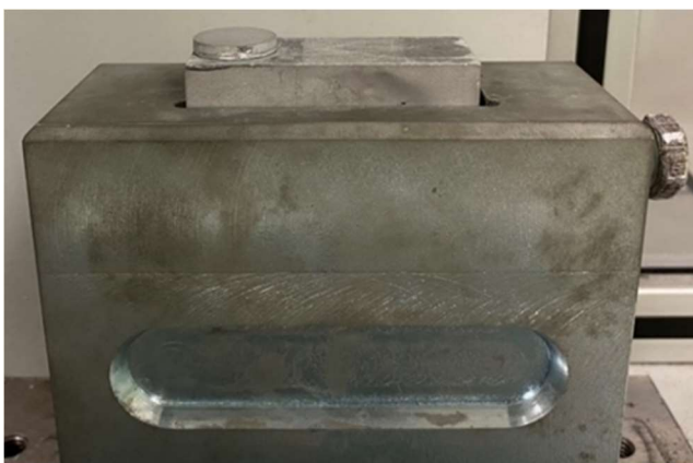
Fig. 5. Sample mounted in the handle of the testing device
