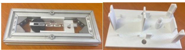
Fig. 6. Universal pallet and preparation for handling
