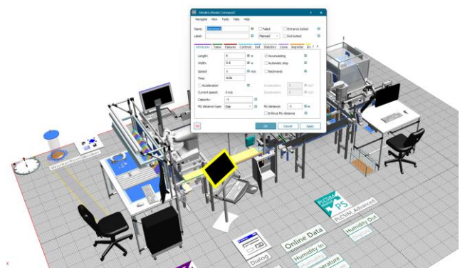
Fig. 4. Setting the conveyor's basic parameters
