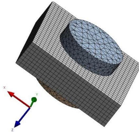
Fig. 7. Grid of elements of the analyzed specimen
