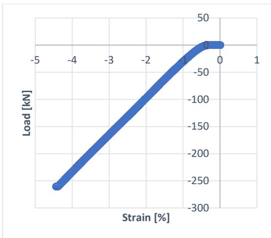
Fig. 2. Compression curve of the composite specimen
