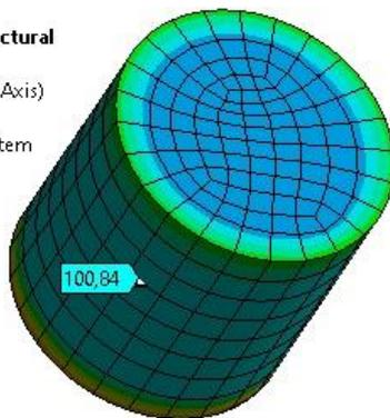
Fig. 8. Normal stresses in the bolt shank of the specimen loaded with a temperature increment of 40°C
