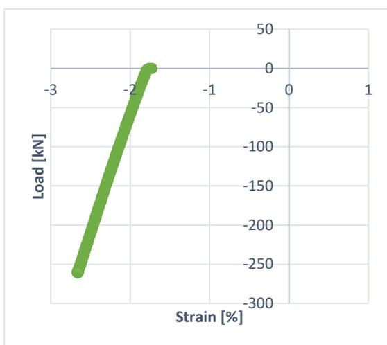
Fig. 3. Stiffness characteristics of the Instron 8802 testing machine
