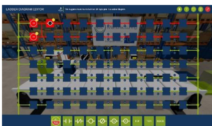
Fig. 3. Virtualization of the ladder diagram programming
