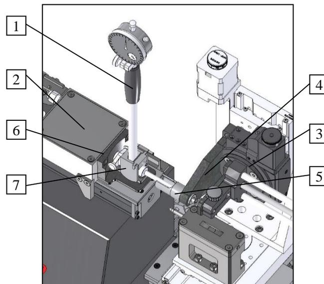
**Fig. 4.** Method for setting a two-point bore gauge with a dial indicator in the device for automatic accuracy inspection of dial indicator readings: 1 – tested bore gauge; 2 – head of the inspection device; 3 – setting module of the inspection device; 4 – bracket; 5 – fixed support element; 6 – movable support element; 7 – bore gauge holder
