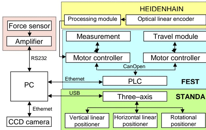
Fig. 5. Diagram of the inspection system structure
