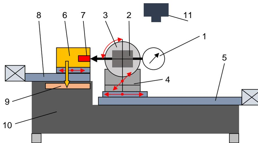
**Fig. 2.** Structural diagram of the measuring instrument inspection system: 1 – tested measuring instrument, 2 – instrument holder, 3 – precision rotary module, 4 – precision linear manipulator (transverse/vertical), 5 – adjustment linear module (longitudinal), 6 – head with measurement base, 7 – force sensor, 8 – precision linear module, 9 – optical measurement scale, 10 – granite body of the inspection device, 11 – camera
