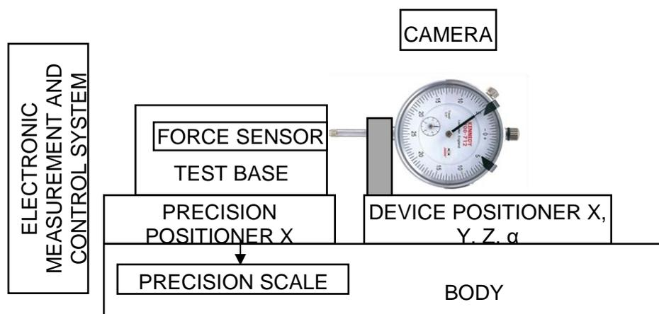
Fig. 1. Diagram of the modular functional system of the inspection system
