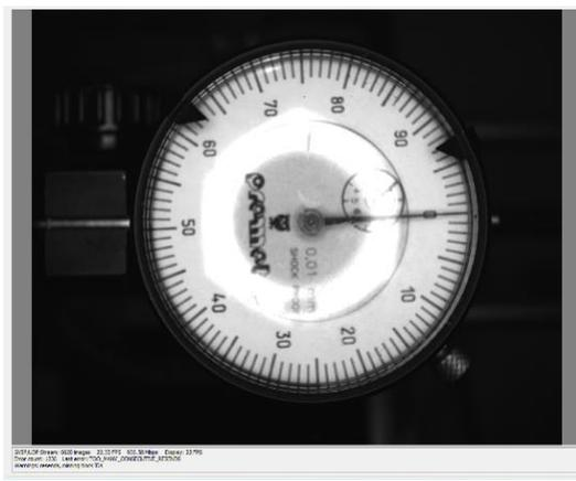
**Fig. 8.** Prototype of the inspection device – use of the camera to ensure precision of dial indicator's readings
