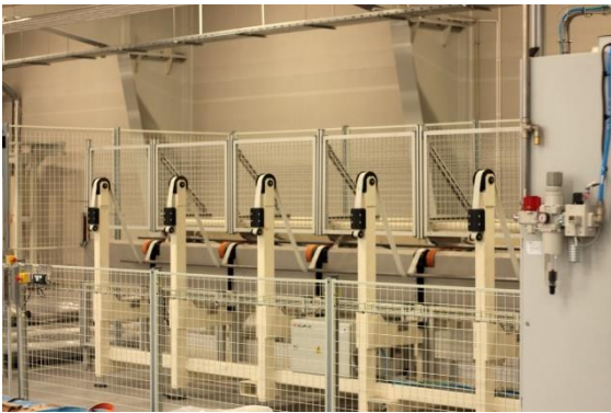
Fig. 6. Tube feeder synchronized with cutting station
