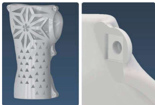
Fig. 5. Front (left photo) and close-up of the place for square nut (right photo) of the 3D model for screws
