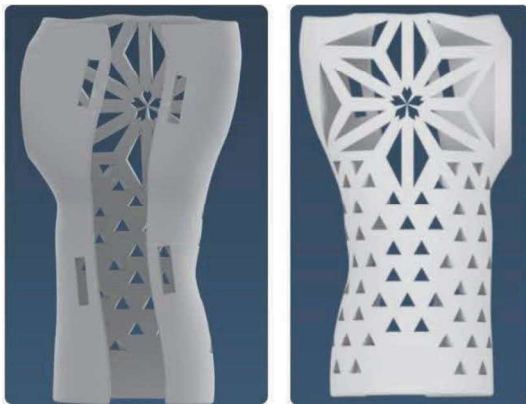
Fig. 4. Back (left photo) and front (right photo) of the 3D model for velcro fastenings
