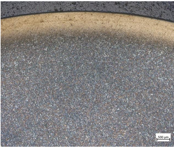
Fig. 4. Image of the cross-section after complex heat treatment with carburizing of steel 16MnCr5 (12.5x magnification)
