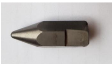
Fig. 2. Photo of burnishing element from cemented carbide G10
