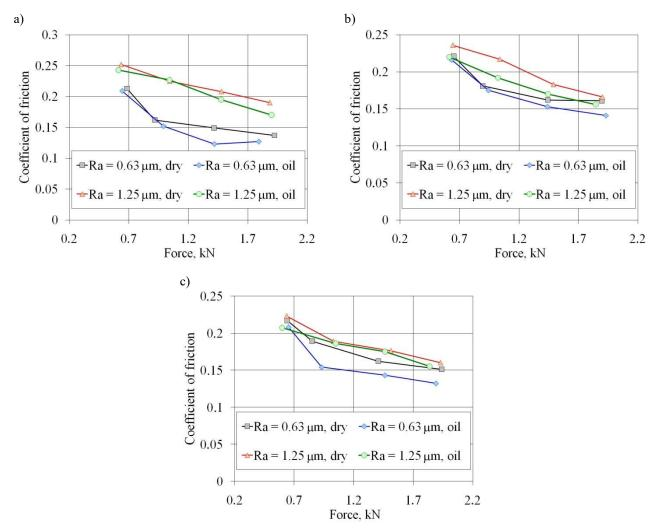
Fig. 6. Effect of force  $F_N$  on the value of coefficient of friction for pre-strained sheets a)  $\phi = 0.095$ , b)  $\phi = 0.139$  and c)  $\phi = 0.182$
