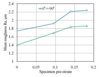
Fig. 5. Effect of specimen pre-strain on the value of mean roughness measured at rolling direction (0°) and transverse to the rolling direction (90°)
