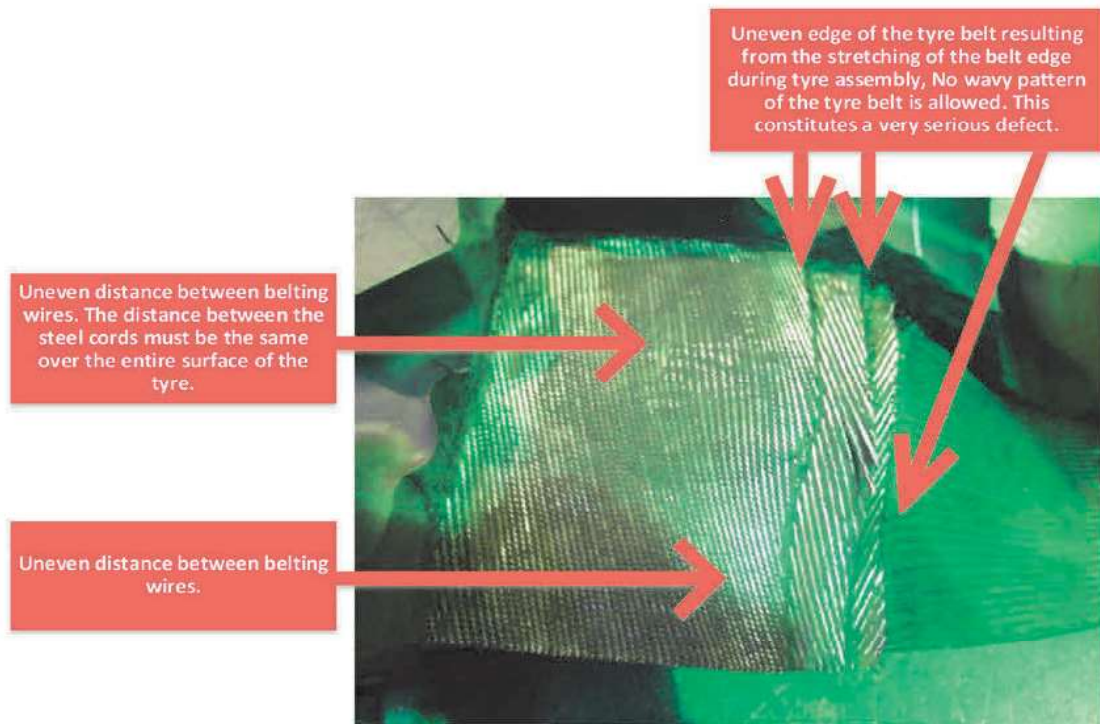
Fig. 5. Example of exceeding the tensile strength limit during the assembly of tyre belt elements [own elaboration]
