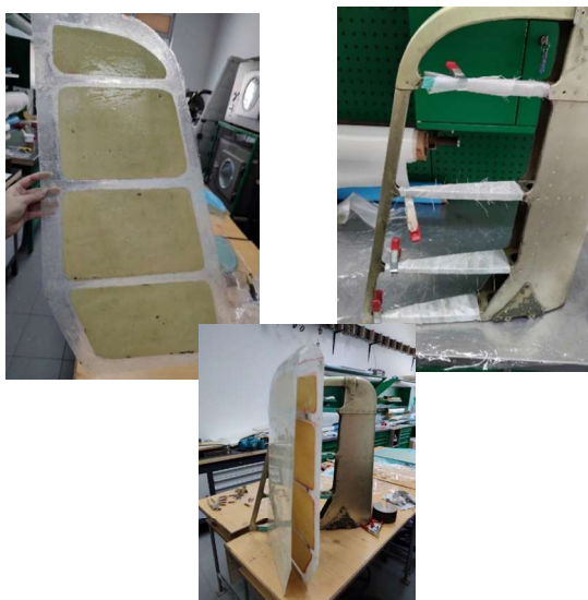
Fig. 2. The top plate of the stabilizer cover and the interior of the new stabilizer cover [Photo S. Tkaczuk]
