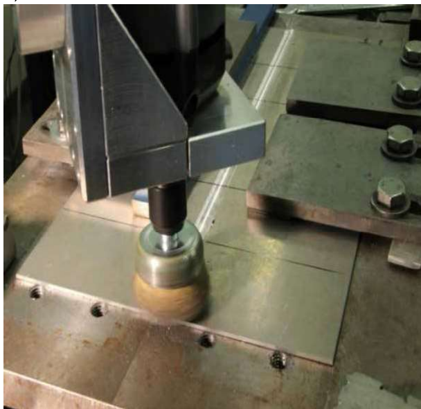
Fig. 1. Brushing with using of: wire brush (a) and brush with ceramic fibres (Xebec) (b)
