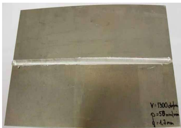
Fig. 8. The view of welded specimen before (a) and after brushing (b)
