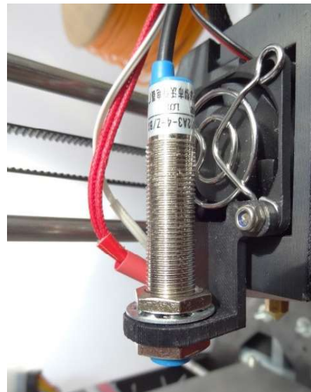
Fig. 8. The holder, the mounting and location of the inductive sensor relative to the extruder nozzle [own elaboration]
