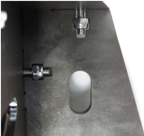
Fig. 3. The assembly method with the use of M3 self-locking screws and nuts, P3Steel printer frame [own elaboration]
