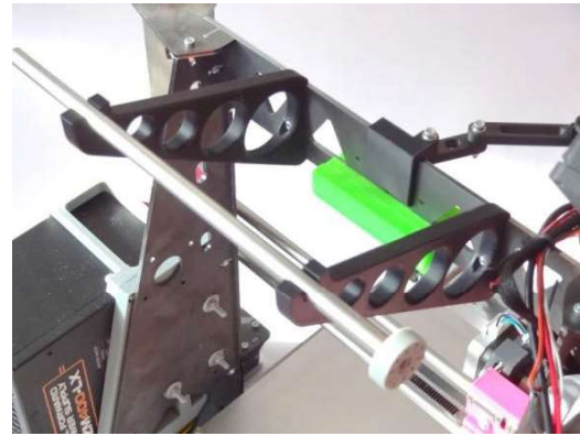
Fig. 7. The mounted holders for the spool of printer raw material [own elaboration]
