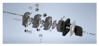
Fig. 4. 3D cam switch model
