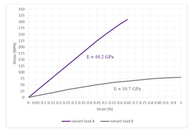
**Fig. 10.** Curves  $\sigma = \sigma(\varepsilon)$  of composite No. 3
