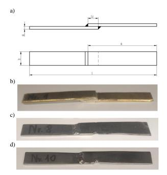
**Fig. 2.** Welded joints: a) diagram of the lap welded joint with double weld used in the tests, b) made of copper alloy, c) made of unalloyed structural steel, d) made of acid-resistant steel
