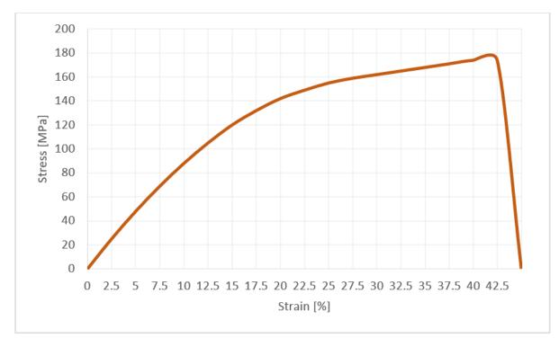
Fig. 11. Curve  $\sigma = \sigma(\varepsilon)$  of composite No. 3 in the load variant B in the entire range of deformations (without using an extension extension extension)
