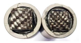
**Fig. 5.** View of the specimen after testing the strength of the composite in the x<sub>3</sub> direction
