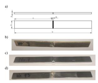
Fig. 1. Welded joints: a) diagram of butt welded joint used in the tests, b) made of copper alloy, c) made of unalloyed structural steel, d) made of acid-resistant steel
