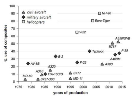
Fig. 1. Mass share of composites in the construction of aircrafts in the years 1975-2015 [5]
