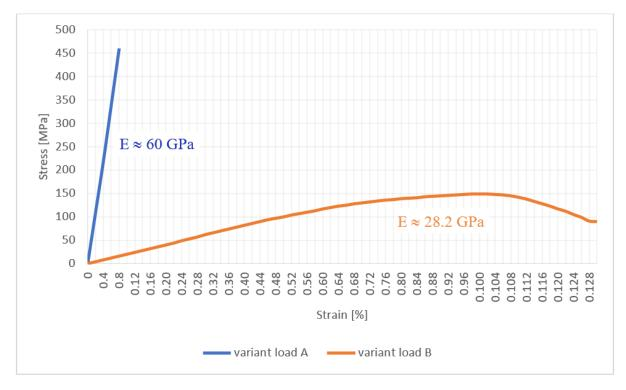
**Fig. 8.** Curves  $\sigma = \sigma(\varepsilon)$  of composite No. 1
