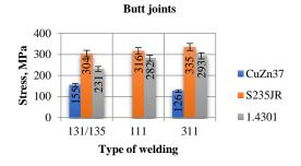
Fig. 3. Stress of butt welded joints
