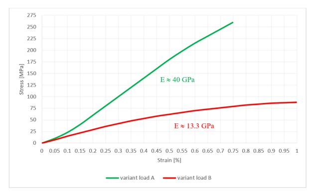
**Fig. 9.** Curves  $\sigma = \sigma(\varepsilon)$  of composite No. 2
