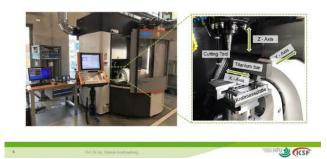
Fig. 10. Experimental setup of cryogenic milling of titanium
