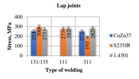
Fig. 4. Stress of lap welded joints
