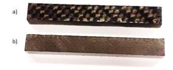
**Fig. 7.** Specimens for impact tests a) in the plane of laying composite layers b) in the cross-sectional plane of the composite
