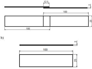
Fig. 2. Scheme of: a) adhesive bond, b) plates for measuring surface roughness
