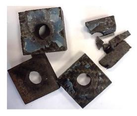
Fig. 13. The form of destruction of a compressed specimen element
