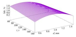
**Fig. 7.** Graph showing the influence of time *t* and ball diameter *d* on the value of the roughness parameter Sdr (p = 0.4 MPa)
