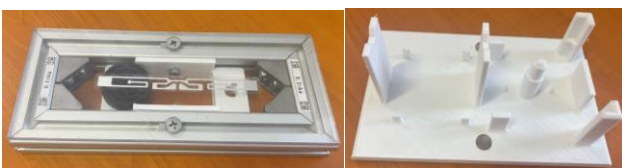
Fig. 6. Universal pallet and preparation for handling
