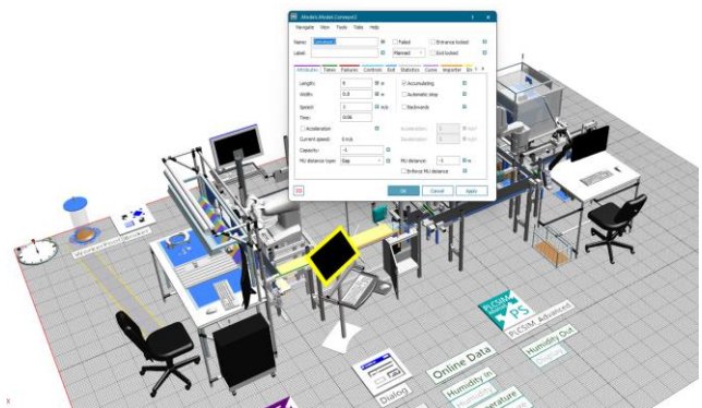
Fig. 4. Setting the conveyor's basic parameters
