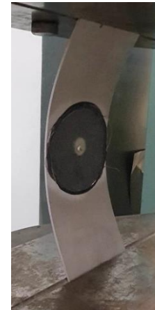
Fig. 5. Specimen loaded with compressive force
