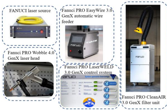
Fig. 3. Construction of a laser welding station
