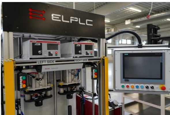
Fig. 16. Leak tester measurement devices
