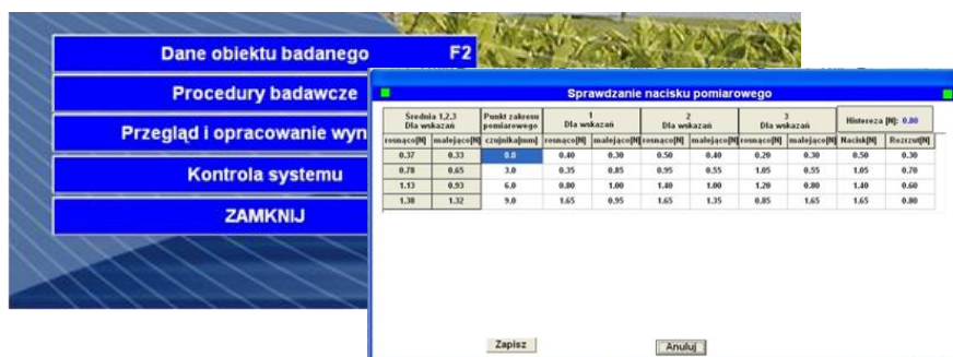
Fig. 6. Sample screens of the control software of the device for monitoring dial indicators (main menu screen and the pressure force check procedure screen)
