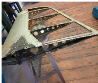
Fig. 1. Stabilizer design [7] [Photo S.Tkaczuk]: 1- cover plate; 2- rib No. 1; 3- rib No. 2; 4- rib No. 3; 5- rib No. 4; 6- rib No. 3; 7- pylon; 8- section; 9- rear strip; 10- metal skin; 11-terminal fairing; 12-truss; 3,14- fabric skin; 15- percale band; 16-countersunk rivet
