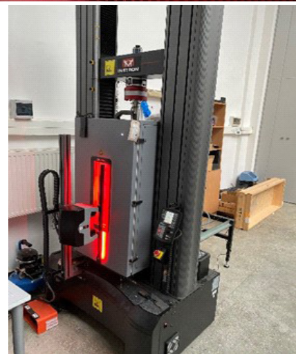
Fig. 2. Strength testing machine with a chamber furnace ready for research
