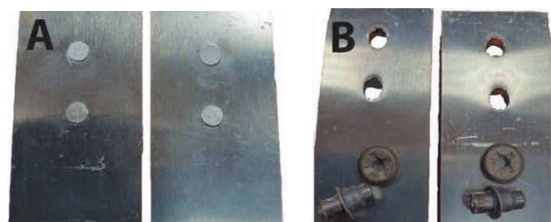
Fig. 2. Destruction of standard and blind rivets in the static strength test
