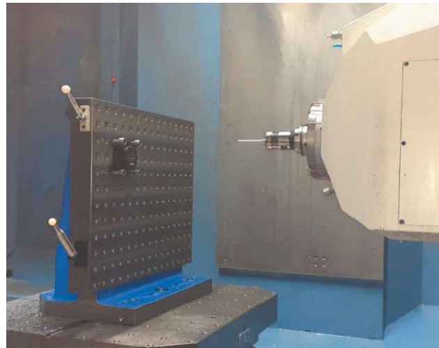
Fig. 7. View of the calibration master (two reference sphere's, calibration column), together with the RMP60 probe, inside 5-axis machine center
