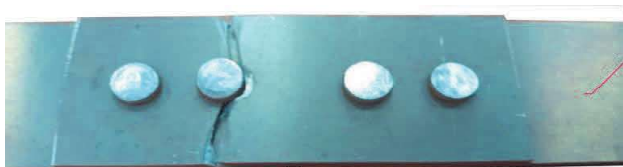
Fig. 11. Fatigue crack of flat cover plate
