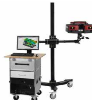
Fig. 4. The measuring stations: a) NIKON iNEXIVE optical coordinate system, b) MarSurf XC20 contact system, c) MCA II measuring arm with the MMDx100 laser head, d) Atos II Triple Scan –structured light
