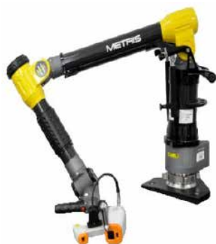
Fig. 4. The measuring stations: a) NIKON iNEXIVE optical coordinate system, b) MarSurf XC20 contact system, c) MCA II measuring arm with the MMDx100 laser head, d) Atos II Triple Scan –structured light
