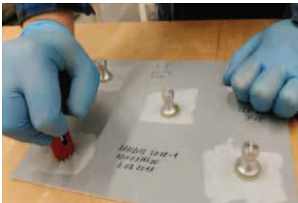
Fig. 1. Removing adhesive outflows Rys. 1. Usuwanie nadmiaru kleju
